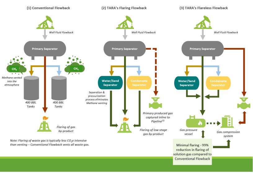
TARA's exclusive Dual Stage Compression System Reduces Carbon Emissions by 99.8%.
