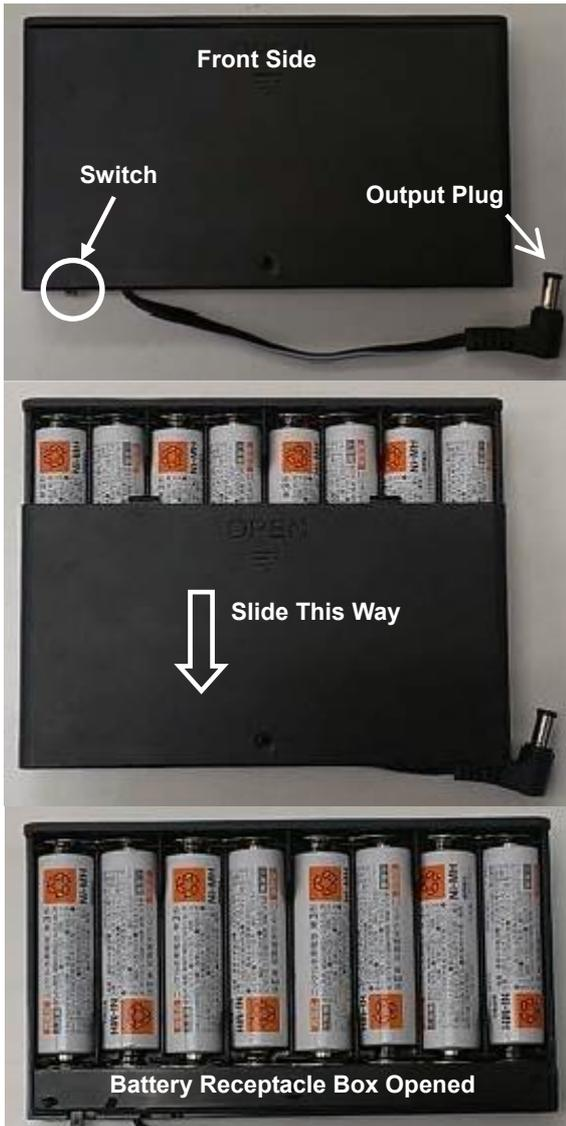
Figure 5-3. Battery Receptacle Box
