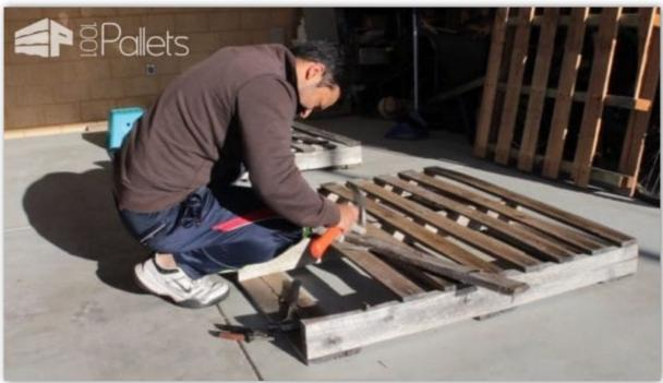
First, you'll need to dismantle one of the two pallets (one pallet for the table and the other one for the chair). For this, I'm using two hammers, but you can check our article to learn how to dismantle a wood pallet in different ways. Also, my goal was to reuse all the nails present in the pallet, so I'll save them and keep them aside when dismantling the pallet.
