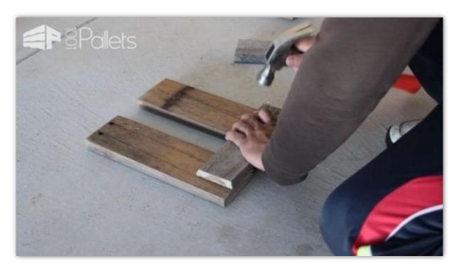
Once the legs are ready, assemble the sitting area. Take the example of the table as the building process is the same one. Then, join the legs to the sitting area as shown in the picture below.
