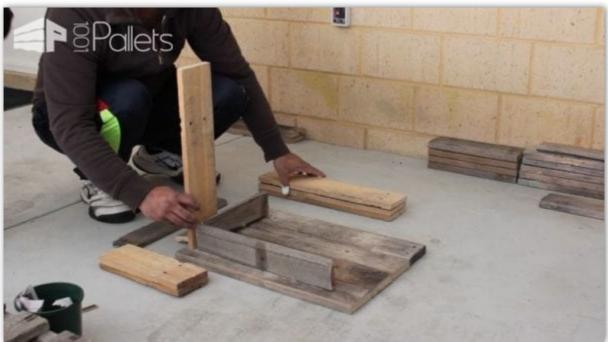
Using a handsaw or a power saw and by following the proper measurements of the table you want, you'll have to cut all the wood that is required to build this kids table. For info, it took me approximately an hour to have all the pieces ready.
